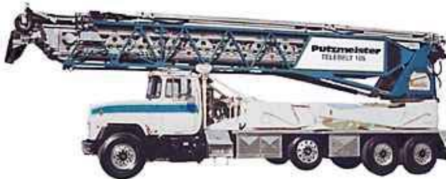
Picture 7. The Putzmeister TB 105 Telebelt
